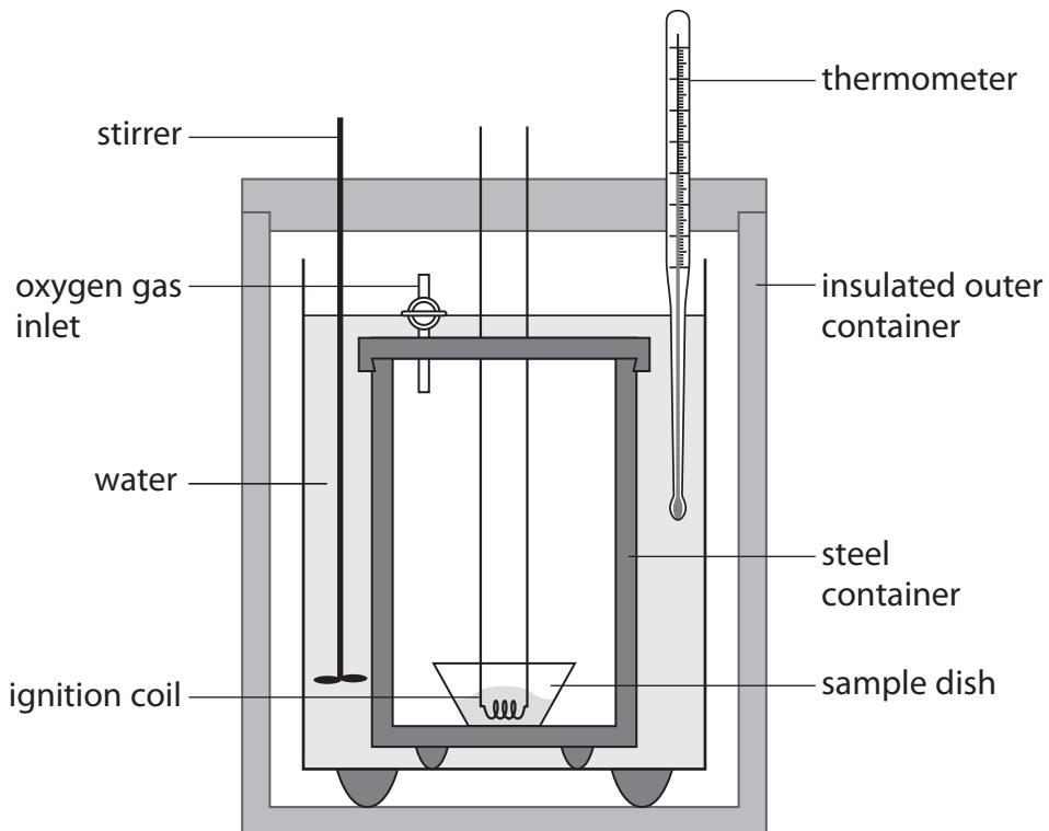
Food is placed in the dish and burnt in air with high levels of oxygen.
