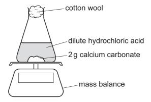
In experiment 1, the calcium carbonate is powdered and an excess of hydrochloric acid is used.
