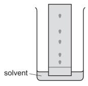
The solvent front is allowed to reach the top of the paper before the chemist removes the paper from the solvent.
