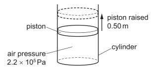
The expansion of the air causes the piston to rise through a vertical distance of 0.50 m, doing 11 kJ of work. Frictional forces are negligible.
