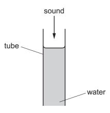
Water is then removed from the tube until a second louder sound is heard.
