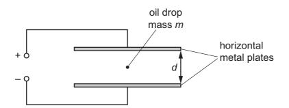
When the potential difference (p.d.) between the plates is  $V_1$  the oil drop rises at a constant speed. When the p.d. is decreased to a value  $V_2$  the oil drop falls at the same constant speed.
