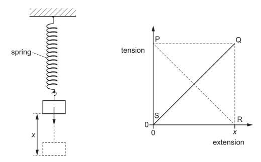
The variation of the tension in the spring with its extension is shown on the graph.
