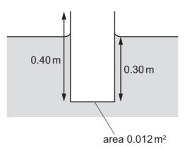
The cross-sectional area of the pipe is  $0.012 \text{ m}^2$ . The weight of the pipe is 32 N.
