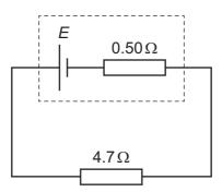
The maximum power that can be dissipated by the resistor without overheating is 0.50 W.
