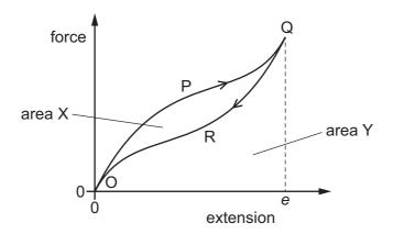
As the force is increased, the curve follows the path OPQ to extension *e*. As the force is reduced, the curve follows the path QRO to return to zero extension.
