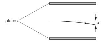
The vertical deflection *x* is measured at the right-hand edge of the plates.
