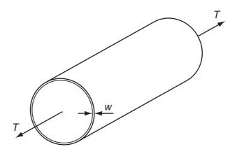
The tube is under tension, caused by a force T, parallel to the axis of the tube. To reduce the stress in the material of the tube, it is proposed to thicken the wall.
