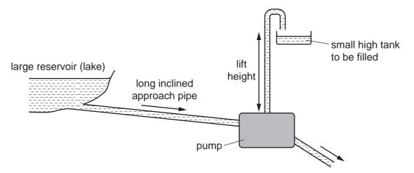
In one such pump the long approach pipe holds 500 kg of water. A valve shuts when the speed of this water reaches  $2.0 \text{ m s}^{-1}$  and the kinetic energy of this water is used to lift a small quantity of water by a height of 15 m.
