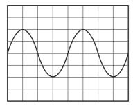
The time-base on the oscilloscope is set to 4 ms/cm.
