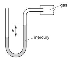
The pressure of the atmosphere is  $p_0$  and the density of mercury is  $\rho$ .
