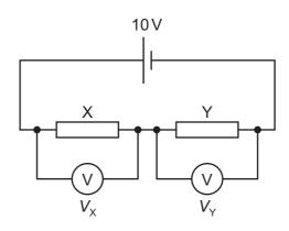
What is the difference  $V_Y - V_X$  of the voltages shown on the voltmeters?
